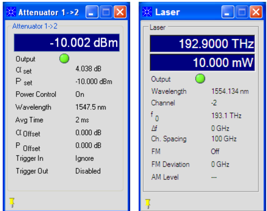
Figure 36 Viewing the measurement on a single channel attenuator/power meter (left) or tunable laser (right)
